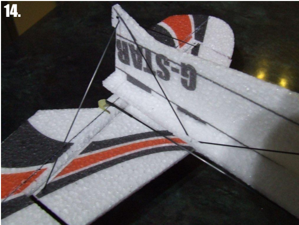
14. Glue on the tailplane, check for alignment, then attach the 1mm bracing.
