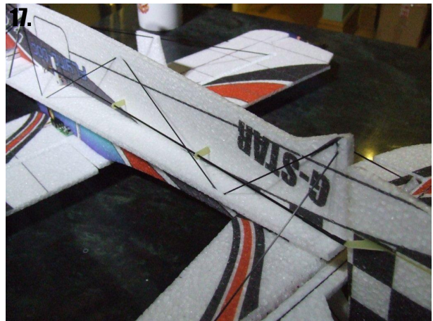
17. Equally space each guide, cutting a slit for each in the foam. Check that the pushrods move freely and are straight, then fix guides to the fuselage with CA.
