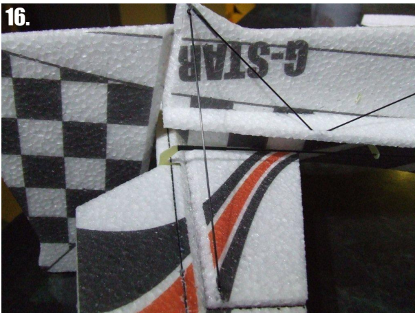
16. Elevator/rudder pushrod assembly. Carbon cut to align with the hinge line and heatshrink to horn. Remember to slide the guides on first.
