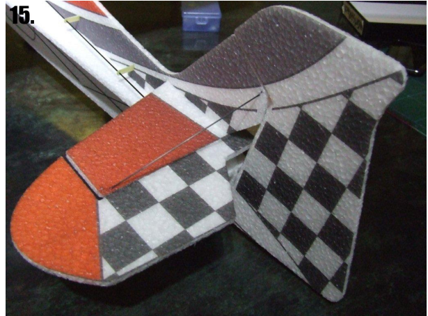
15. Attach the rudder and upper 1mm bracing.
