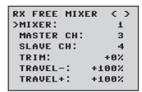
Up to five mixers can be contemporaneously programmed. You can switch between Mixer 1, Mixer 2, 3, 4 ... and mixer 5 in the "Mixer" line
